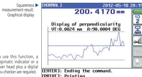
To use this function, a Digimatic indicator or a lever head plus a digital Mu-checker are required.
